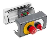
design means that when an enclosure is opened, the wiring is pulled out with the lid of the box. With ABB's design, the blocks and wiring stays neatly in place when the lid is removed, even if the enclosure has been already been mounted. This makes maintenance, rewiring, light bulb changes, and contact rearrangement super-simple.
