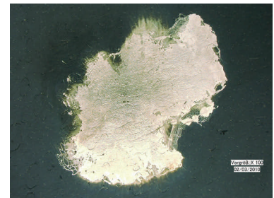
Self-healing event in typical metalized film
