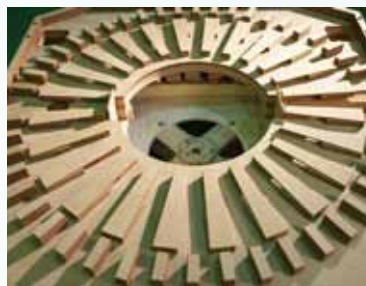
Construction of Oil Duct
