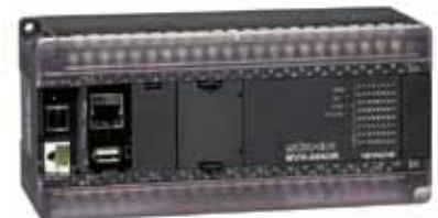
MICRO-EHV I/O line ups : 40/64 points Program Memory : 16 ksteps Processing Speed: 0.3 \mu s Built-in Communications Port: USB Port (for programmng) Serial Port (RS232C), USB memory port, Ethernet
