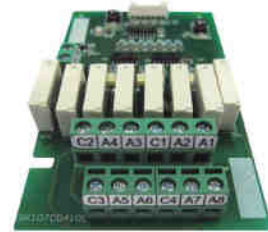
WS01 Fan and water pump Multi-channel control board
