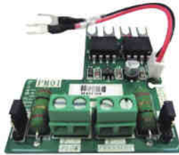
PM01 Injection molding machine specific expansion board
