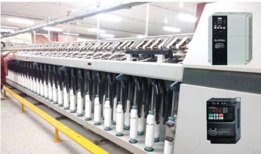
Textile Machine Driven by Hitachi Inverter
